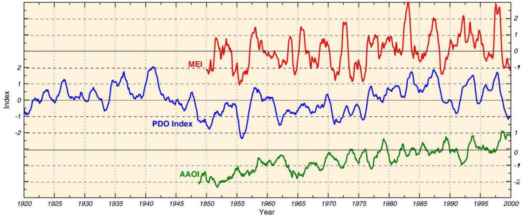
**Fig. 5.** Time series (1920–2000) of monthly mean Multivariate ENSO Index (MEI), PDO Index and AAO Index. All indexes were smoothed using a 5-month running mean filter. Original indices obtained from Climate Diagnostic Center (NOAA).
